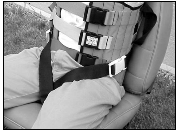
Figure 11 - Leg Strap Applied In "Criss-Cross" Configuration
