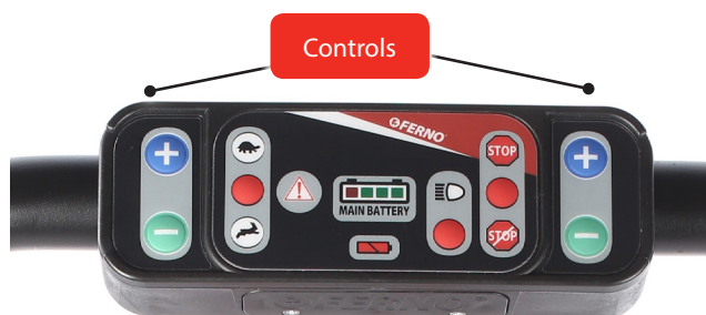
Figure 10 - Ascent and descent controls
