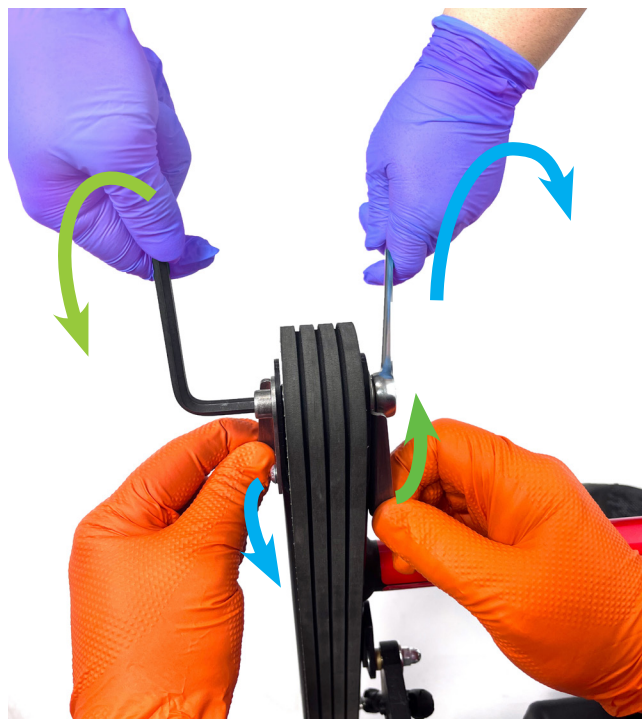
Figure 50 - Adjusting track tension.
