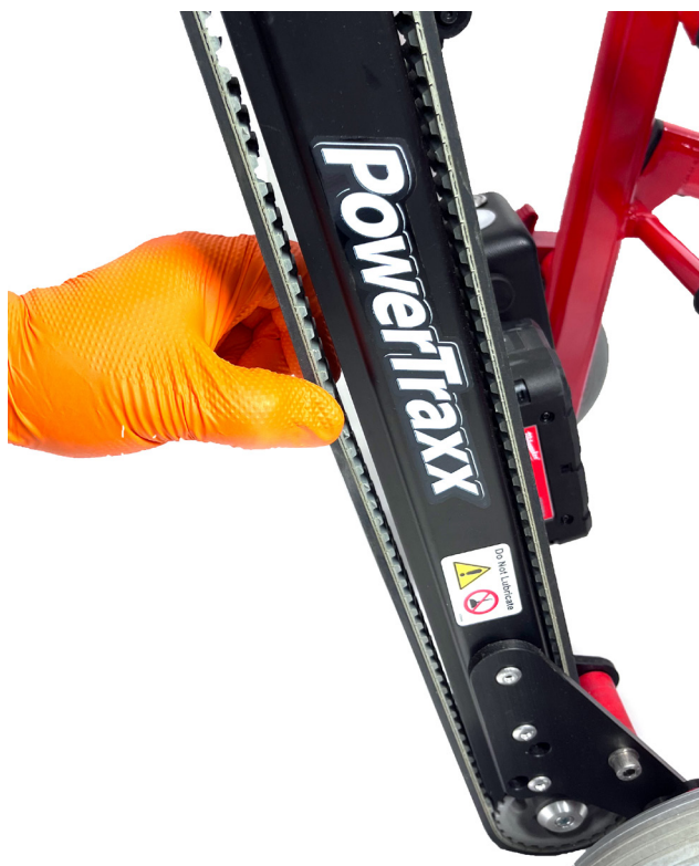
Figure 52 - Checking track tension.
