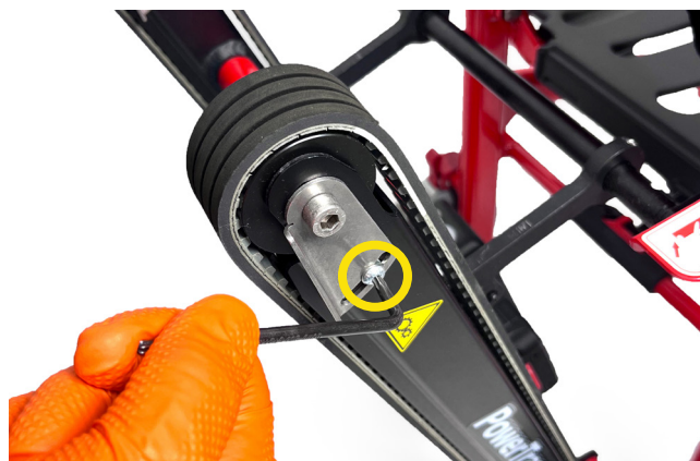
Figure 51 - Adjusting track tension.
