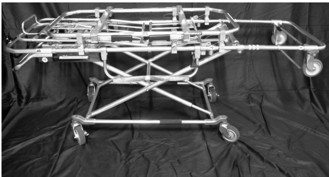
Figure 14: Installation of ITC-HL frame on Ferno 35A Stretcher.
