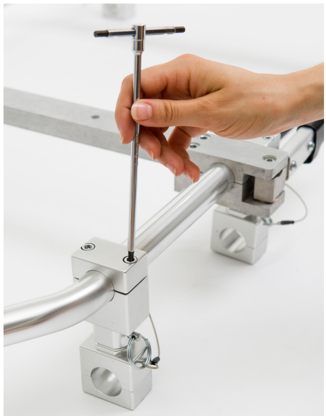
Figure 4: Assembly of fixed block on ITC-HL frame.
