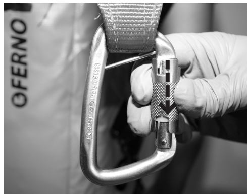
Figure 5 - Push gate barrel away (downward) from strap end of karabiner
