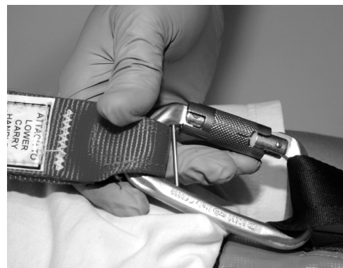
Figure 8 - On release of karabiner gate, the unit automatically closes and locks
